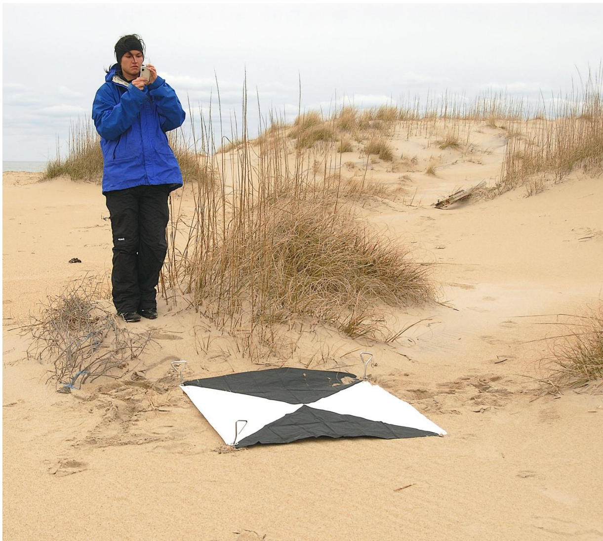
Figure 10. Aerial target used for the lighthouse camera rectification. Photograph by Don Bowers.
